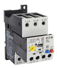
Eaton XT series electronic overload relay, 0.33-1.65A adjustable, solid state, stand-alone power connection(s), DIN rail or panel mount. For use with any contactor.
