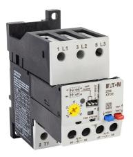
Eaton XT series electronic overload relay, 9.0-45.0A adjustable, solid state, stand-alone power connection(s), DIN rail or panel mount. For use with any contactor.
