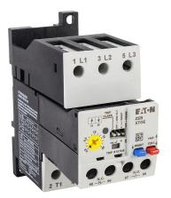
Eaton XT series electronic overload relay, 4.0-20.0A adjustable, solid state, ground fault protection, stand-alone power connection(s), DIN rail or panel mount. For use with any contactor.
