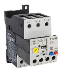
Eaton XT series electronic overload relay, 1.0-5.0A adjustable, solid state, stand-alone power connection(s), DIN rail or panel mount. For use with any contactor.
