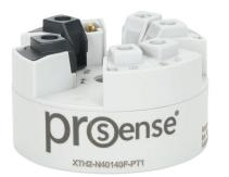
ProSense temperature transmitter, non-isolated, Pt100 RTD input, -40 to 140 deg F fixed, 4-20 mA output, 10-36 VDC operating voltage, DIN Form B connection head mount, screw terminals.
