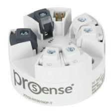
ProSense temperature transmitter, isolated, Input: 1-channel, Type T thermocouple, -100 to 100 deg F fixed, Output: 1-channel, output current signal range(s) of 4-20 mA, 10-36 VDC operating voltage, DIN Form B connection head mount, screw terminals.
