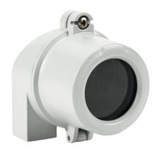
ProSense field housing, (2) 1/2in female NPT, -40 to +100 degrees C (-40 to 212 degrees F), aluminum, NEMA 4X, IP66 IP68. For use with programmable temperature transmitter XTH2-0-UNV-S and XTH2-0-UNV-P.
