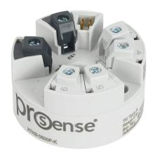
ProSense temperature transmitter, isolated, Input: 1-channel, Type K thermocouple, 0 to 800 deg F fixed, Output: 1-channel, output current signal range(s) of 4-20 mA, 10-36 VDC operating voltage, DIN Form B connection head mount, screw terminals.
