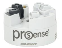
ProSense temperature transmitter, non-isolated, Pt100 RTD input, 0 to 500 deg F fixed, 4-20 mA output, 10-36 VDC operating voltage, DIN Form B connection head mount, screw terminals.
