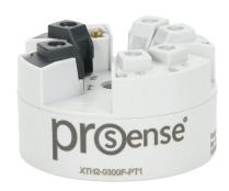
ProSense temperature transmitter, non-isolated, Pt100 RTD input, 0 to 300 deg F fixed, 4-20 mA output, 10-36 VDC operating voltage, DIN Form B connection head mount, screw terminals.
