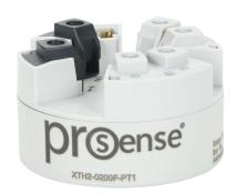
ProSense temperature transmitter, non-isolated, Pt100 RTD input, 0 to 200 deg F fixed, 4-20 mA output, 10 to 36 VDC operating voltage, DIN Form B connection head mount, screw terminals.
