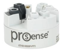
ProSense temperature transmitter, non-isolated, Pt100 RTD input, 0 to 200 deg F fixed, 4-20 mA output, 10-36 VDC operating voltage, DIN Form B connection head mount, screw terminals.
