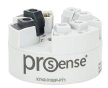
ProSense temperature transmitter, non-isolated, Pt100 RTD input, 0 to 100 deg F fixed, 4-20 mA output, 10 to 36 VDC operating voltage, DIN Form B connection head mount, screw terminals.
