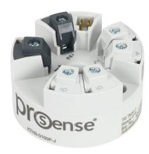
ProSense temperature transmitter, isolated, Input: 1-channel, Type J thermocouple, 0 to 100 deg F fixed, Output: 1-channel, output current signal range(s) of 4-20 mA, 10-36 VDC operating voltage, DIN Form B connection head mount, screw terminals.
