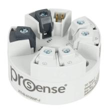
ProSense temperature transmitter, isolated, Input: 1-channel, Type J thermocouple, 0 to 1000 deg F fixed, Output: 1-channel, output current signal range(s) of 4-20 mA, 10-36 VDC operating voltage, DIN Form B connection head mount, screw terminals.
