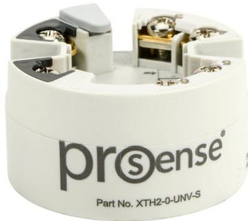
ProSense programmable temperature transmitter, isolated, RTD, thermocouple, millivolt or potentiometer input, deg F or deg C, current output, 10-36 VDC operating voltage, DIN Form B connection head mount, screw terminals.
