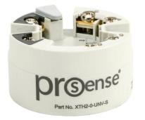
ProSense programmable temperature transmitter, isolated, RTD, thermocouple, millivolt or potentiometer input, deg F or deg C, current output, 10-36 VDC operating voltage, DIN Form B connection head mount, screw terminals.
