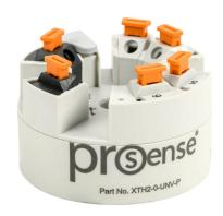
ProSense programmable temperature transmitter, isolated, RTD, thermocouple, millivolt or potentiometer input, deg F or deg C, current output, 10-36 VDC operating voltage, DIN Form B connection head mount, push-in terminals.
