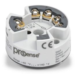
ProSense temperature transmitter, isolated, Pt100 RTD input, -40 to 140 deg F fixed, 4-20 mA output, 8-35 VDC operating voltage, DIN Form B connection head mount, screw terminals.
