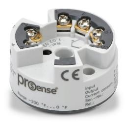
ProSense temperature transmitter, isolated, Type T thermocouple input, -200 to 0 deg F fixed, 4-20 mA output, 8-35 VDC operating voltage, DIN Form B connection head mount, screw terminals.
