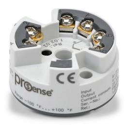
ProSense temperature transmitter, isolated, Type T thermocouple input, -100 to 100 deg F fixed, 4-20 mA output, 8 to 35 VDC operating voltage, DIN Form B connection head mount, screw terminals.
