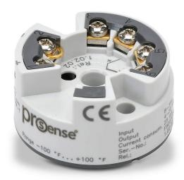
ProSense temperature transmitter, isolated, Type T thermocouple input, -100 to 100 deg F fixed, 4-20 mA output, 8-35 VDC operating voltage, DIN Form B connection head mount, screw terminals.
