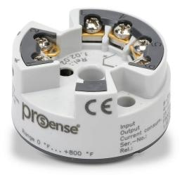
ProSense temperature transmitter, isolated, Input: 1-channel, Type K thermocouple, 0 to 800 deg F fixed, Output: 1-channel, output current signal range(s) of 4-20 mA, 8-35 VDC operating voltage, DIN Form B connection head mount, screw terminals.
