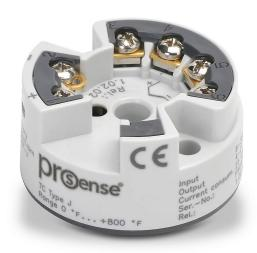
ProSense temperature transmitter, isolated, Type J thermocouple input, 0 to 800 deg F fixed, 4-20 mA output, 8-35 VDC operating voltage, DIN Form B connection head mount, screw terminals.
