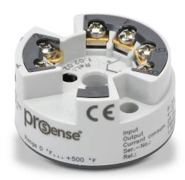
ProSense temperature transmitter, isolated, Type K thermocouple input, 0 to 500 deg F fixed, 4-20 mA output, 8 to 35 VDC operating voltage, DIN Form B connection head mount, screw terminals.
