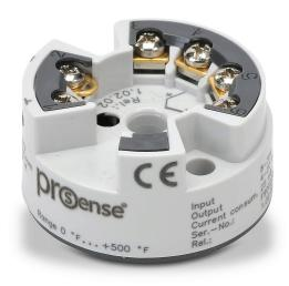
ProSense temperature transmitter, isolated, Type K thermocouple input, 0 to 500 deg F fixed, 4-20 mA output, 8-35 VDC operating voltage, DIN Form B connection head mount, screw terminals.
