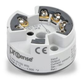
ProSense temperature transmitter, isolated, Pt100 RTD input, 0 to 300 deg F fixed, 4-20 mA output, 8 to 35 VDC operating voltage, DIN Form B connection head mount, screw terminals.
