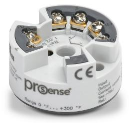
ProSense temperature transmitter, isolated, Type K thermocouple input, 0 to 300 deg F fixed, 4-20 mA output, 8-35 VDC operating voltage, DIN Form B connection head mount, screw terminals.
