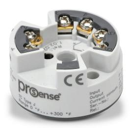
ProSense temperature transmitter, isolated, Type J thermocouple input, 0 to 300 deg F fixed, 4-20 mA output, 8-35 VDC operating voltage, DIN Form B connection head mount, screw terminals.
