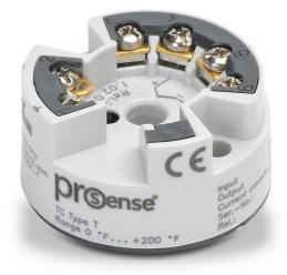
ProSense temperature transmitter, isolated, Type T thermocouple input, 0 to 200 deg F fixed, 4-20 mA output, 8-35 VDC operating voltage, DIN Form B connection head mount, screw terminals.
