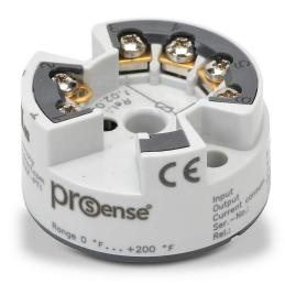
ProSense temperature transmitter, isolated, Pt100 RTD input, 0 to 200 deg F fixed, 4-20 mA output, 8-35 VDC operating voltage, DIN Form B connection head mount, screw terminals.
