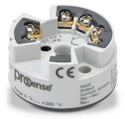
ProSense temperature transmitter, isolated, Type K thermocouple input, 0 to 200 deg F fixed, 4-20 mA output, 8-35 VDC operating voltage, DIN Form B connection head mount, screw terminals.
