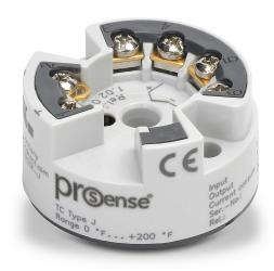
ProSense temperature transmitter, isolated, Type J thermocouple input, 0 to 200 deg F fixed, 4-20 mA output, 8-35 VDC operating voltage, DIN Form B connection head mount, screw terminals.
