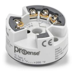
ProSense temperature transmitter, isolated, Type J thermocouple input, 0 to 200 deg F fixed, 4-20 mA output, 8 to 35 VDC operating voltage, DIN Form B connection head mount, screw terminals.
