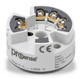
ProSense temperature transmitter, isolated, Type K thermocouple input, 0 to 2000 deg F fixed, 4-20 mA output, 8-35 VDC operating voltage, DIN Form B connection head mount, screw terminals.
