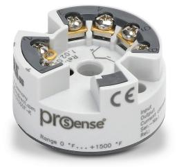
ProSense temperature transmitter, isolated, Type K thermocouple input, 0 to 1500 deg F fixed, 4-20 mA output, 8-35 VDC operating voltage, DIN Form B connection head mount, screw terminals.
