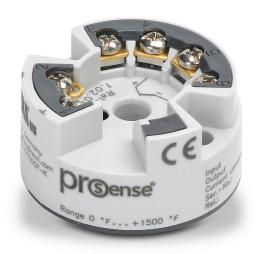
ProSense temperature transmitter, isolated, Type K thermocouple input, 0 to 1500 deg F fixed, 4-20 mA output, 8 to 35 VDC operating voltage, DIN Form B connection head mount, screw terminals.
