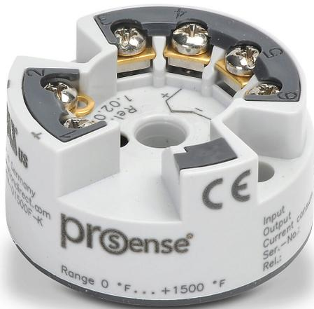
ProSense temperature transmitter, isolated, Type K thermocouple input, 0 to 1500 deg F fixed, 4-20 mA output, 8-35 VDC operating voltage, DIN Form B connection head mount, screw terminals.
