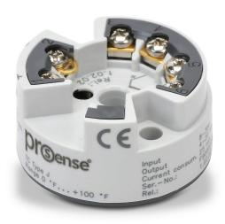
ProSense temperature transmitter, isolated, Type J thermocouple input, 0 to 100 deg F fixed, 4-20 mA output, 8-35 VDC operating voltage, DIN Form B connection head mount, screw terminals.
