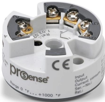
ProSense temperature transmitter, isolated, Type K thermocouple input, 0 to 1000 deg F fixed, 4-20 mA output, 8-35 VDC operating voltage, DIN Form B connection head mount, screw terminals.
