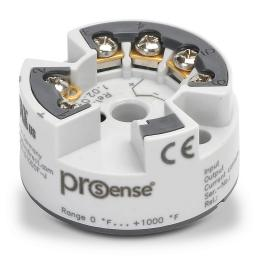
ProSense temperature transmitter, isolated, Type J thermocouple input, 0 to 1000 deg F fixed, 4-20 mA output, 8-35 VDC operating voltage, DIN Form B connection head mount, screw terminals.
