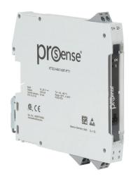
ProSense temperature transmitter, non-isolated, Input: 1-channel, Pt100 RTD, -40 to 140 deg F fixed, Output: 1-channel, output current signal range(s) of 4-20 mA, 10-36 VDC operating voltage, 35mm DIN rail mount, removable screw terminal plugs.
