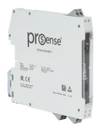
ProSense temperature transmitter, isolated, Input: 1-channel, Type T thermocouple, -100 to 100 deg F fixed, Output: 1-channel, output current signal range(s) of 4-20 mA, 10-36 VDC operating voltage, 35mm DIN rail mount, removable screw terminal plugs.
