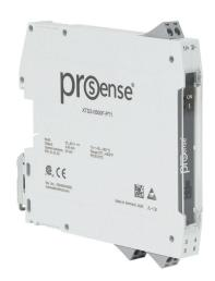
ProSense temperature transmitter, non-isolated, Input: 1-channel, Pt100 RTD, 0 to 500 deg F fixed, Output: 1-channel, output current signal range(s) of 4-20 mA, 10-36 VDC operating voltage, 35mm DIN rail mount, removable screw terminal plugs.
