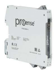
ProSense temperature transmitter, isolated, Input: 1-channel, Type K thermocouple, 0 to 500 deg F fixed, Output: 1-channel, output current signal range(s) of 4-20 mA, 10-36 VDC operating voltage, 35mm DIN rail mount, removable screw terminal plugs.
