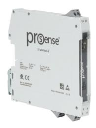
ProSense temperature transmitter, isolated, Input: 1-channel, Type J thermocouple, 0 to 500 deg F fixed, Output: 1-channel, output current signal range(s) of 4-20 mA, 10-36 VDC operating voltage, 35mm DIN rail mount, removable screw terminal plugs.
