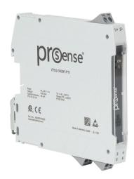
ProSense temperature transmitter, non-isolated, Input: 1-channel, Pt100 RTD, 0 to 300 deg F fixed, Output: 1-channel, output current signal range(s) of 4-20 mA, 10-36 VDC operating voltage, 35mm DIN rail mount, removable screw terminal plugs.
