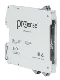
ProSense temperature transmitter, isolated, Input: 1-channel, Type K thermocouple, 0 to 200 deg F fixed, Output: 1-channel, output current signal range(s) of 4-20 mA, 10-36 VDC operating voltage, 35mm DIN rail mount, removable screw terminal plugs.
