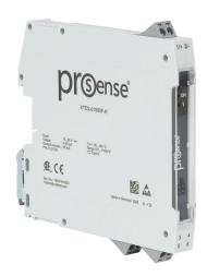
ProSense temperature transmitter, isolated, Input: 1-channel, Type K thermocouple, 0 to 1500 deg F fixed, Output: 1-channel, output current signal range(s) of 4-20 mA, 10-36 VDC operating voltage, 35mm DIN rail mount, removable screw terminal plugs.
