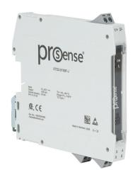
ProSense temperature transmitter, isolated, Input: 1-channel, Type J thermocouple, 0 to 100 deg F fixed, Output: 1-channel, output current signal range(s) of 4-20 mA, 10-36 VDC operating voltage, 35mm DIN rail mount, removable screw terminal plugs.
