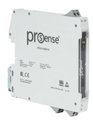
ProSense temperature transmitter, isolated, Input: 1-channel, Type K thermocouple, 0 to 1000 deg F fixed, Output: 1-channel, output current signal range(s) of 4-20 mA, 10-36 VDC operating voltage, 35mm DIN rail mount, removable screw terminal plugs.
