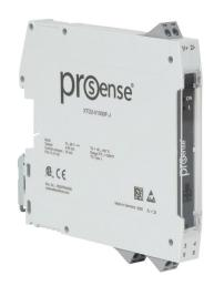
ProSense temperature transmitter, isolated, Input: 1-channel, Type J thermocouple, 0 to 1000 deg F fixed, Output: 1-channel, output current signal range(s) of 4-20 mA, 10-36 VDC operating voltage, 35mm DIN rail mount, removable screw terminal plugs.
