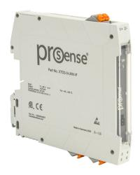
ProSense programmable temperature transmitter, isolated, RTD, thermocouple, millivolt or potentiometer input, deg F or deg C, current output, 11-36 VDC operating voltage, 35mm DIN rail mount, removable push-in terminal plugs.
