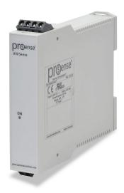
ProSense temperature transmitter, isolated, Type T thermocouple input, -200 to 0 deg F fixed, 4-20 mA output, 12 to 35 VDC operating voltage, 35mm DIN rail mount, removable screw terminal plugs.
