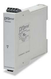
ProSense temperature transmitter, isolated, Type T thermocouple input, -200 to 0 deg F fixed, 4-20 mA output, 12-35 VDC operating voltage, 35mm DIN rail mount, removable screw terminal plugs.
