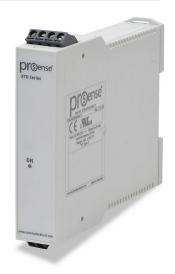
ProSense temperature transmitter, isolated, Type T thermocouple input, -100 to 100 deg F fixed, 4-20 mA output, 12 to 35 VDC operating voltage, 35mm DIN rail mount, removable screw terminal plugs.
