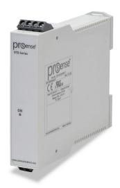
ProSense temperature transmitter, isolated, Type T thermocouple input, -100 to 100 deg F fixed, 4-20 mA output, 12-35 VDC operating voltage, 35mm DIN rail mount, removable screw terminal plugs.
