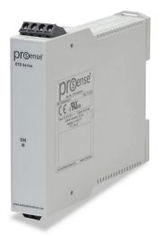
ProSense temperature transmitter, isolated, Type K thermocouple input, 0 to 800 deg F fixed, 4-20 mA output, 12-35 VDC operating voltage, 35mm DIN rail mount, removable screw terminal plugs.
