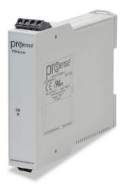
ProSense temperature transmitter, isolated, Type K thermocouple input, 0 to 800 deg F fixed, 4-20 mA output, 12 to 35 VDC operating voltage, 35mm DIN rail mount, removable screw terminal plugs.
