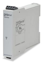
ProSense temperature transmitter, isolated, Type J thermocouple input, 0 to 800 deg F fixed, 4-20 mA output, 12-35 VDC operating voltage, 35mm DIN rail mount, removable screw terminal plugs.
